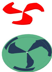
Ionetix Upgraded CS-30 Magnet Sector Shims
