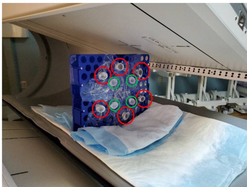
Figure 2. Limit of detection phantom scanned by the Optima 640 gamma-camera. The six identical conical polypropylene vials are filled with different concentrations of ^{223}\text{Ra} : 74, 37, 27.7, 18.5, 9.2, and 3.7 kBq/mL. The red circles denote the vials containing the hot sources while the green circles denote the vials filled with water.
