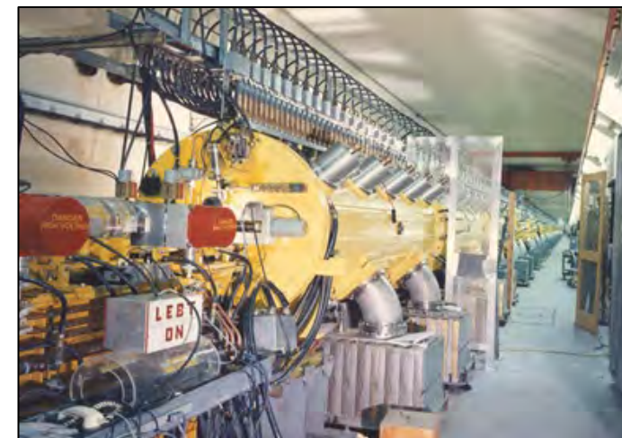
BNL Linac at the Brookhaven Linac Isotope Producer (BLIP) 165 \mu\text{A} intensity to targets at incident energies ranging from 66-202 MeV
