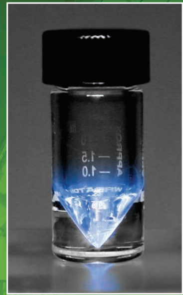
Actinium-225 final product, with blue glow due to phosphorescence of the glass vial by alpha particles.
