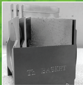
Target stack assembly used for the BNL/ORNL 100 mCi batch.
