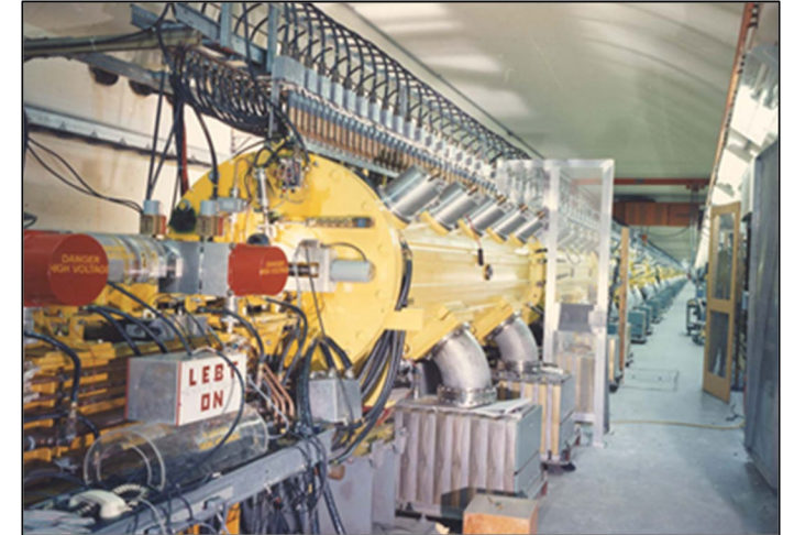
BNL Linac at the Brookhaven Linac Isotope Producer (BLIP) 165 \mu\text{A} intensity to targets at incident energies ranging from 66-202 MeV
