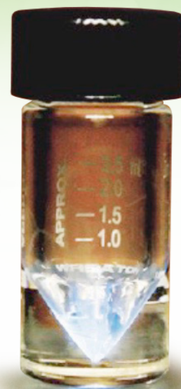
Actinium-225 final product, with blue glow from ionization of surrounding air by alpha particles
