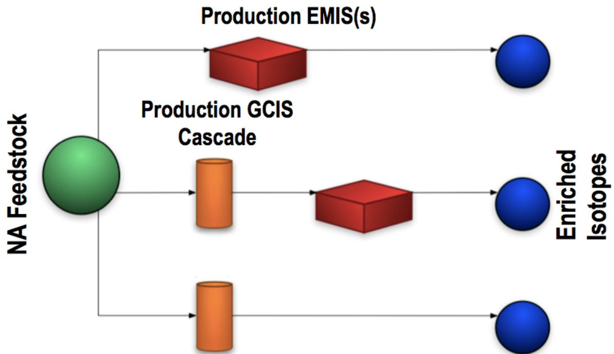
ORNL Proposed Production Scheme for the prototype Enriched Stable Isotope Production Facility (NA: natural abundance, EMIS: Electromagnetic Isotope Separator, GCIS: Gas Centrifuge Isotope Separator).
