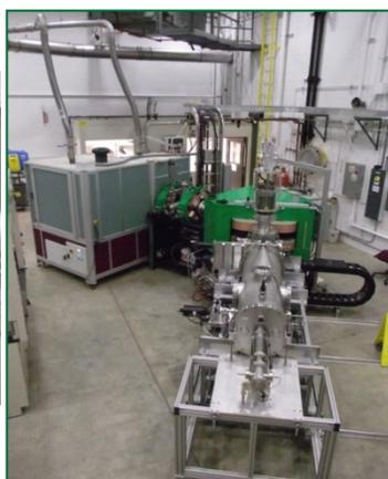
**Pictures of the ORNL R&D EMIS. Experimental enrichment trials have been conducted and efforts to increase ion current (throughput) are ongoing.**
