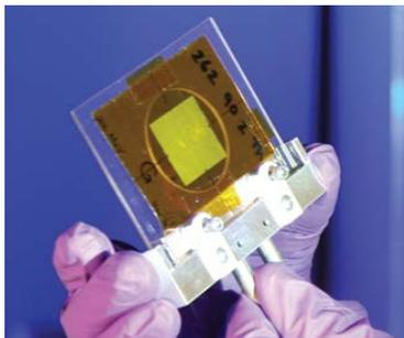
**Thorium test foil target used to measure cross sections for proton production of Ac-225.**
