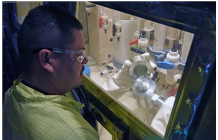
Packaging of Am-241 in LANL glovebox. (Image courtesy of LANL.)
