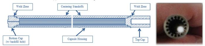
New high-specific activity Co-60 target axial cross-section (left)); top view (right) showing multi-channel loading feature that enables increased production.
