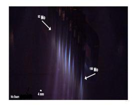
Picture of the isotope collection pockets during a molybdenum separation. Separated ion beams are focused into the graphite lined collection pockets.
