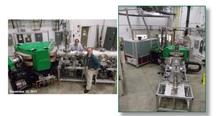
Pictures of the ORNL R&D EMIS. Experimental enrichment trials have been conducted and efforts to increase ion current (throughput) are ongoing.
